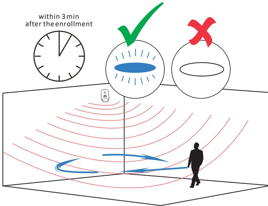
Note: while the detector is disarmed, power off and power on will make the detector enter the walk test mode.
