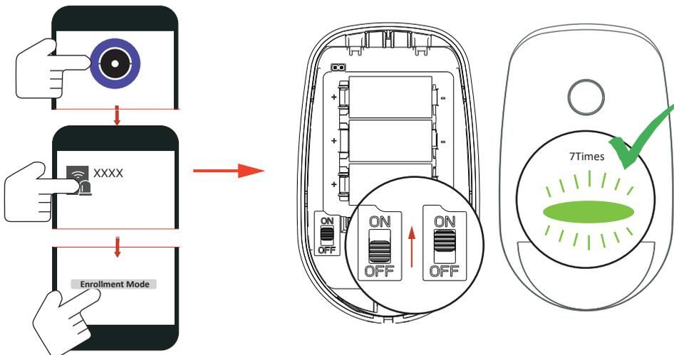
Note: make the device power off, hold the tamper switch and then power on for re-enrollment synchronously.
