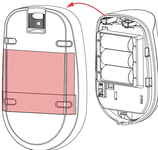
Note: Installing with sponge tape is non EN compliant.
